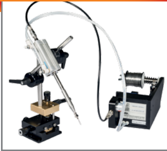
Wire Feeder Dispensers (2)
